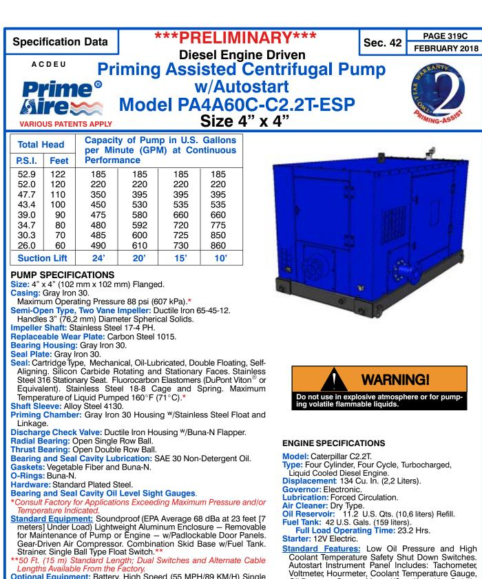
Optional Equipment: Battery. High Speed (55 MPH/89 KM/H) Single Axle Pneumatic-Tired Wheel Kit W/<sub>WO</sub> DOT-Approved Lights and Electric Brakes. Tandem Axle Over-the-Road Trailer (Meets DOT Requirements) Available W/Either Electric or Hydraulic Surge Brakes, Running Lights, Jack Stands and Safety Cables/Chains. EPS W/Submersible Transducer Liquid Level Sensor (50 Ft. [15 M] Cable Standard, Alternate Lengths Available).
