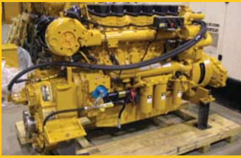
January 2000 Francesca Madre's 2000 C18 package with Twin Disc MG-5114DC gearbox 3.43:1 ratio, rotary oil pump to quickly drain engine and gearbox, and deep oil sump for extended oil change intervals.
