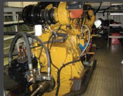
Mated to the C18 engine on the William T.R. is a ZF W350 gearbox with 3.5:1 ratio and a clutchable SAE 'C' PTO to drive a Denison hydraulic pump to power the hydraulic generator. With this configuration the boat's electrical load is provided from the main engine and eliminating the need to operate a separate diesel generator while under way.
