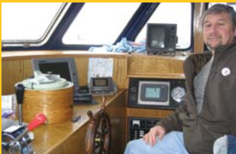
Repower of Vito Figliomeni's (above) Francesca Madre was completed by Frank Baptista and the staff at Hike Metal Products. The existing push/pull cables and levers were re-used and integrated to the new Cat Multi-Station Control Station through the use of a throttle position sensor. During the repower Hike was able to rejuvenate the wheelhouse giving it a beautiful new look. To Vito's right is the Cat Marine Power Display unit that connects to the C18 electronic engine. All essential engine and gearbox information is monitored via the Marine Power Display.
