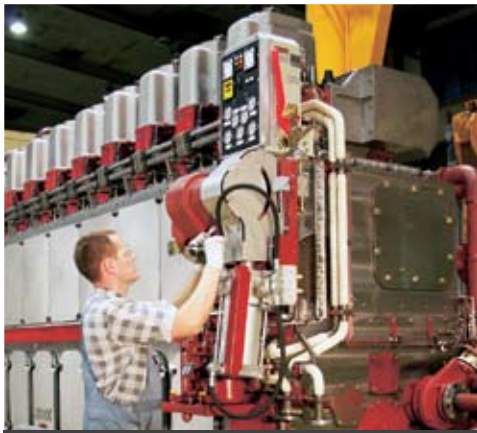
FCT Unit mounted on a MaK 8M 32C LEE Marine Engine
